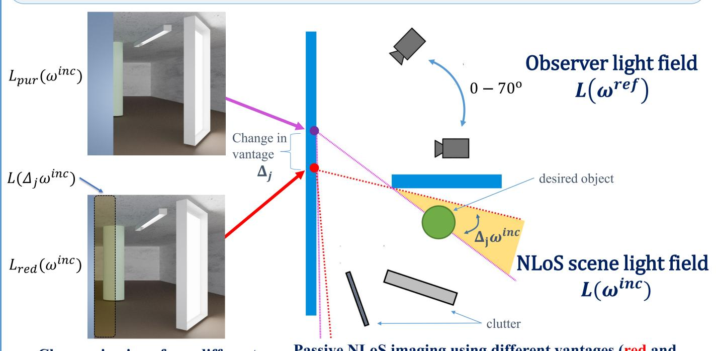
Passive NLoS imaging using different vantages (red and Changes in views from different purple) to image object (green) in presence of clutter (gray) vantages due to wall obstruction
