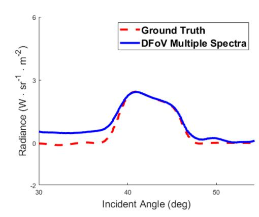
Reconstructed object using multiple-spectra light field
